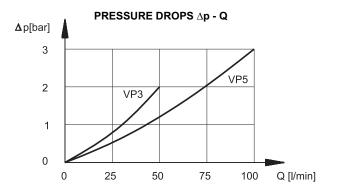
**NOTE:** The curves shown in the graph refer to  $B \rightarrow A$  and  $A \rightarrow B$  flow with the valve released hydraulically.
